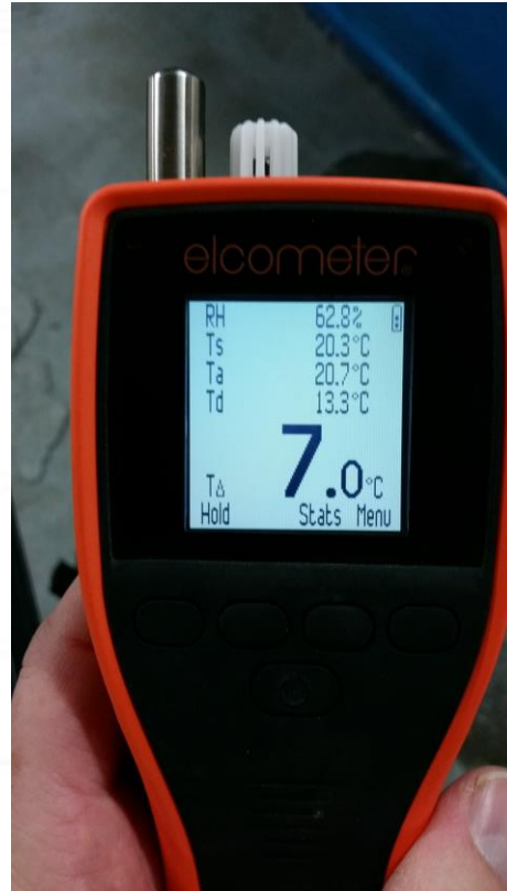
*One of our testing methods prior to floor installation
